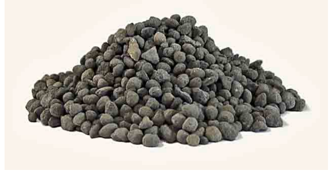
Clinker – raw material for producing Cement
